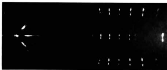
Fig. 10. a -axis 15^\circ -oscillation photograph of the lower part of crystal No. 2. \phi varies from 25^\circ to 40^\circ ; Cu K\alpha radiation; camera radius 3 cm; polytype 4H .
